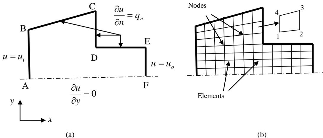
**Fig. 1.** The problem domain and its finite-element representation
