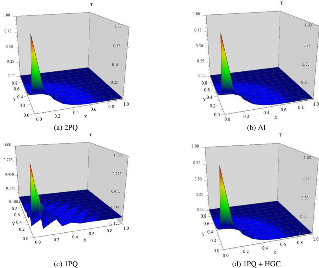
**Fig. 3.** Heat-conduction problem with the boundary condition  $T = 1.0$  at  $(0,0)$ : solutions with (a) 2PQ, (b) AI, (c) 1PQ without HGC and (d) 1PQ with HGC.
