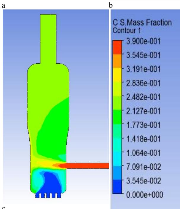
**Fig. 16.** Carbon solid mass fraction contour for a) the base case, b) case one and c) case two
