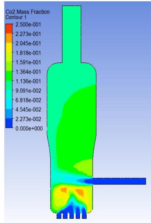
**Fig. 17b.** CO and CO<sub>2</sub> mass fraction contour for case (1) regenerator multiple air inlets
