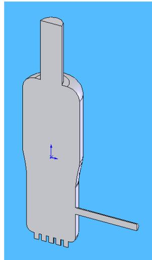
**Fig. 6.** Case (2): multiple air inlets (5 air inlets)  $\phi$ 0.78m, one catalyst inlet 1.1m its axis's raised by 100% 2.5m, outlet catalyst 3.51m
