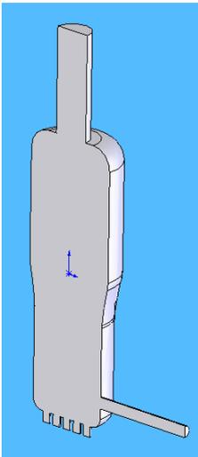
**Fig. 5.** Case (1): multiple air inlets (5 air inlets)  $\phi$ 0.78m, one catalyst inlet 1.1m, one outlet 3.51m
