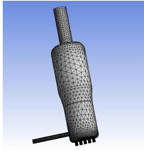
**Fig. 8.** Mesh for case (1) regenerator multiple air inlets
