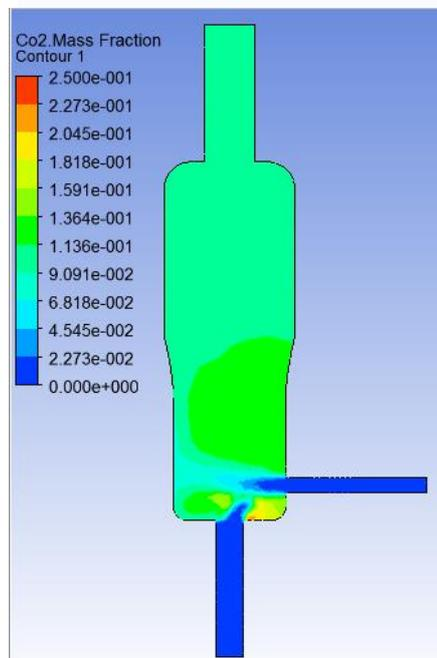
**Fig. 17a.** CO and CO<sub>2</sub> mass fraction contour for base case regenerator single air inlet
