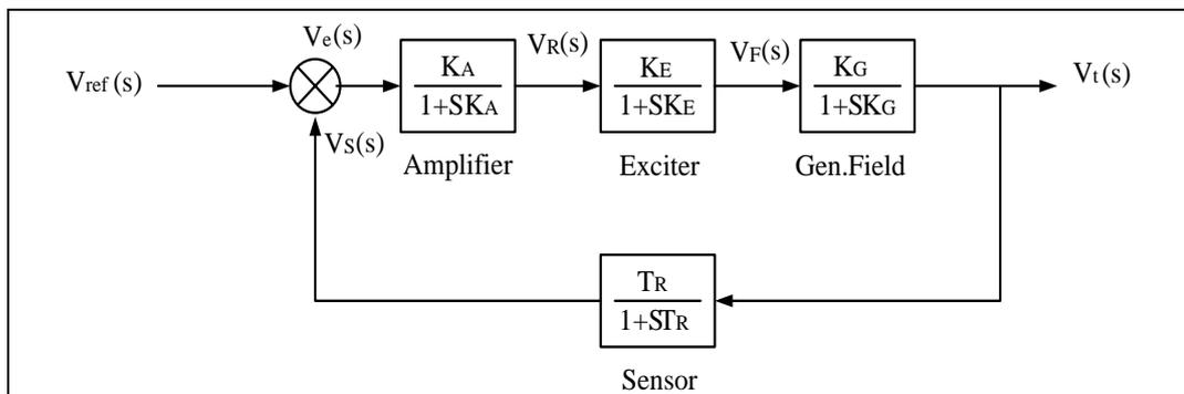
Fig. 4. Automatic voltage regulator models
