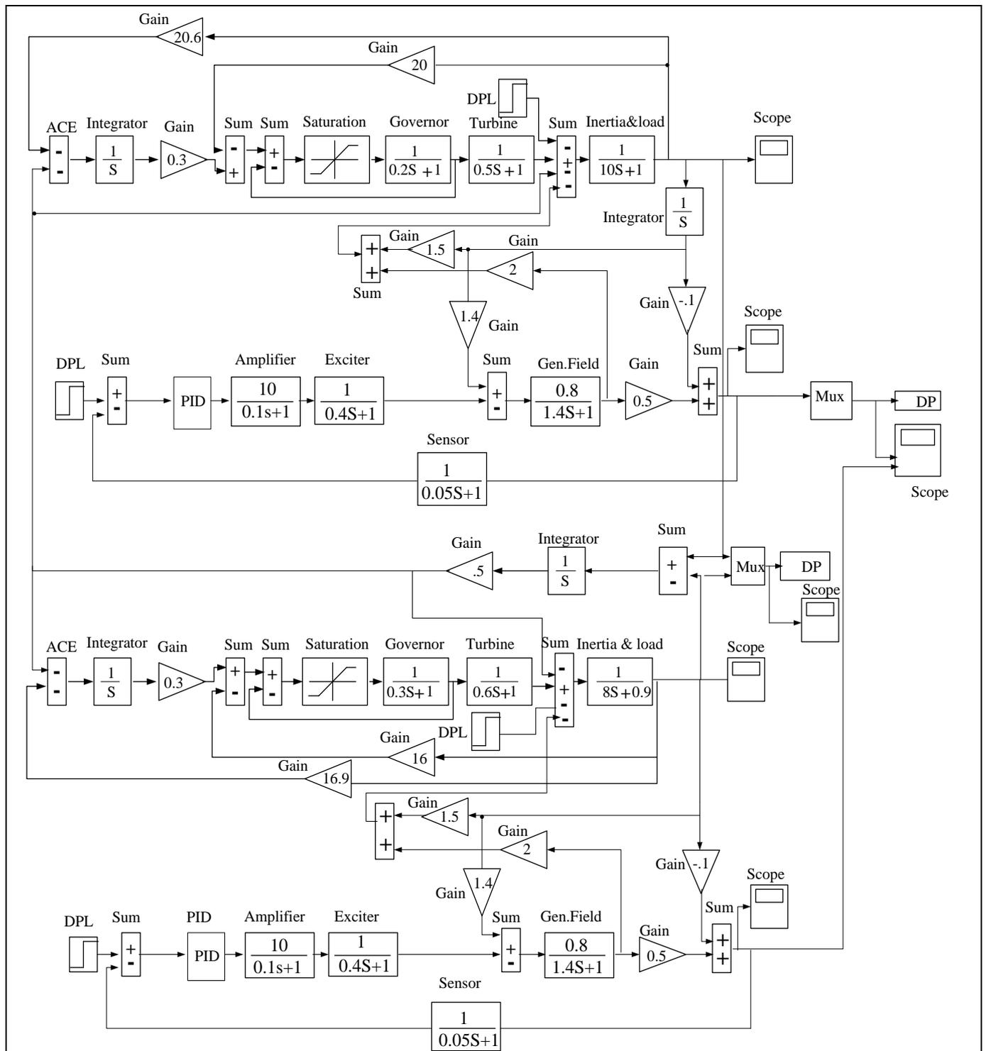
Fig. 11. SIMULINK model of two areas of AGC and AVR considering GRC
