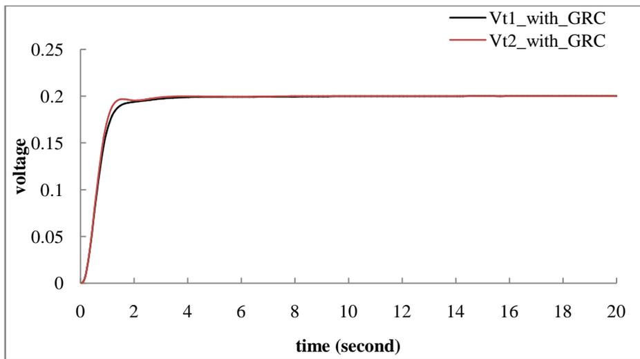
Fig.13. Terminal voltage of two areas AGC, AVR and GRC
