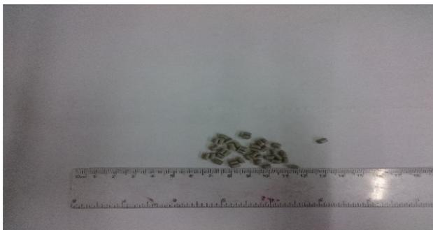
**Figure 2: Recycled PP plastic pellets sample – Tarig Elmahdi for Plastic Pellets Recycling**
