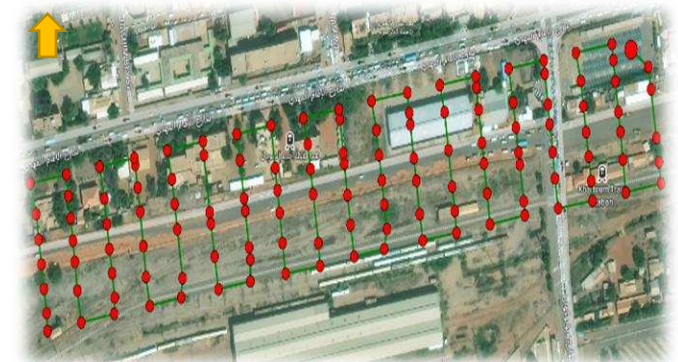
Fig. 3. Flight Plan (camera positions in red).
