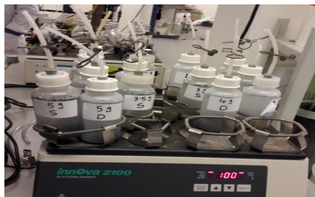
Fig .3. Batch isotherm experiment set-up
