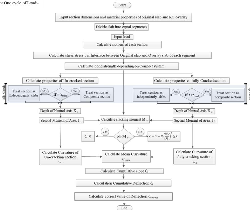
Fig .3. Flowchart of modelling strengthened RC slab using RC overlay
