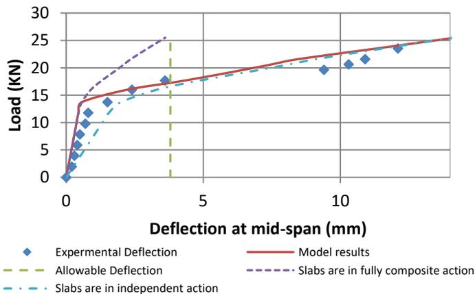
Fig .7. Load-deflection curves of slab 1 (Friction only)
