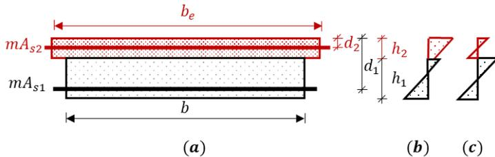
Fig. 2. (a) Equivalent section of strengthened slab; (b) Fully composite action stresses; (c) Independent action stresses.
