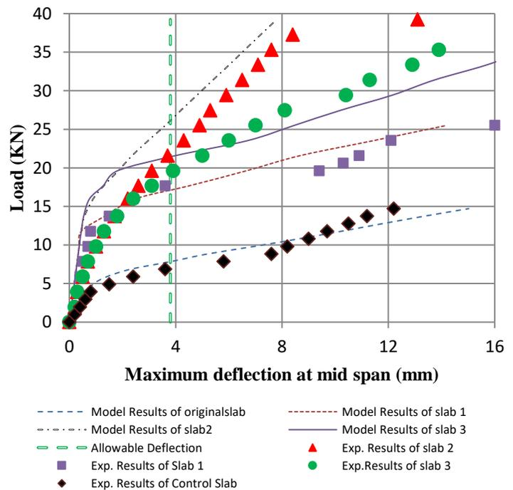
Fig. 11. Load-deflection curve of strengthened slabs compared to the reference slab
