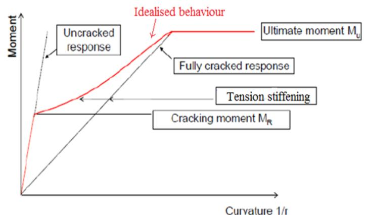
Fig. 1. Typical moment–curvature response
