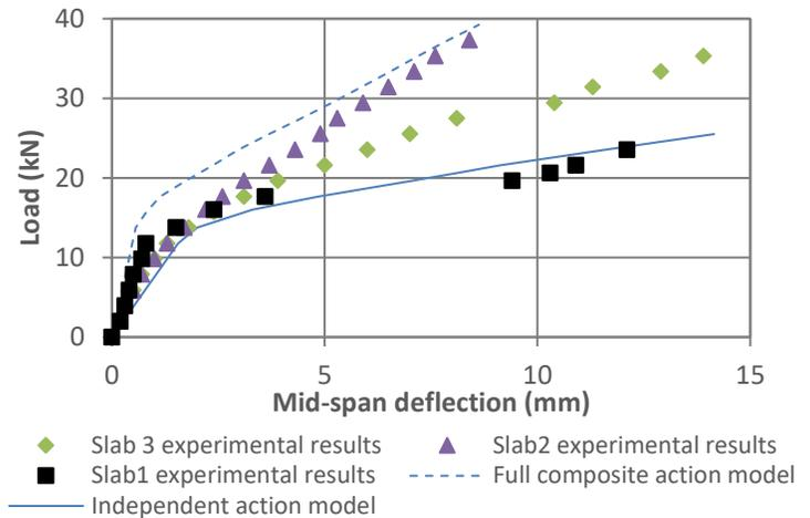
Fig .6. Expected zone of load-deflection curves of strengthened slabs
