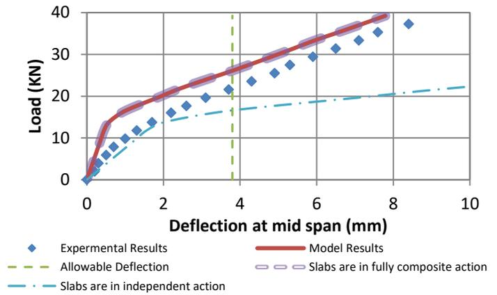
Fig .9. Load-deflection relationship of slab 2 (Epoxy)
