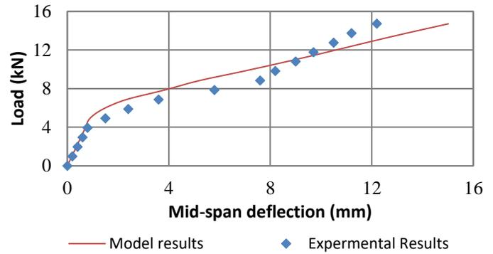
Fig .5. Load-deflection curve of the reference slab
