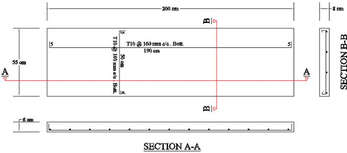
Fig .4. Structural detailing of the original slabs
