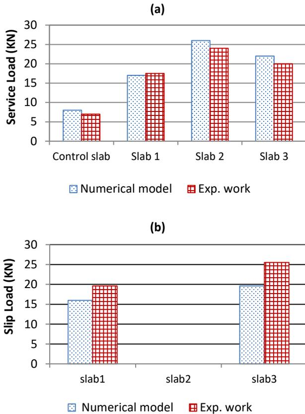
**Fig. 12.** Comparison of slabs in terms of: (a) Service load; (b) Slippage Load
