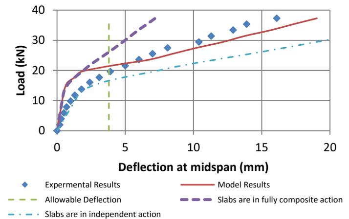
Fig .10. Load-Deflection relationship of slab 3 (Shear keys)
