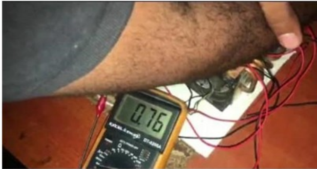
Figure 10: the output voltage of the contact between forearm and the Peltier surface
