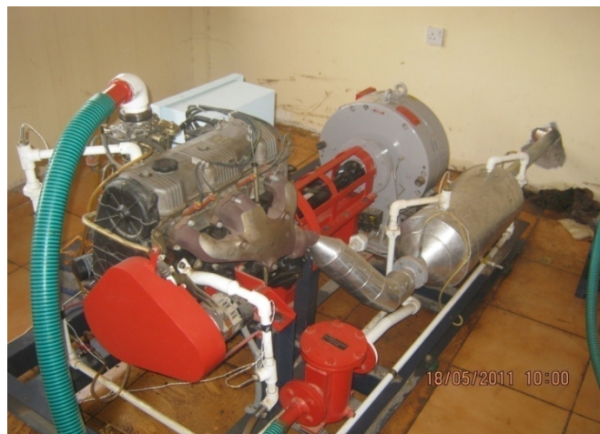
Fig. 1. Engine test rig used for the tested blends
